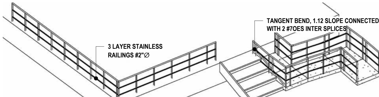
TYPICAL STAIRS & RAILINGS DETAIL
